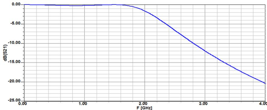
Figure 7. Simulated  $s_{21}$  of constant k low pass filter
