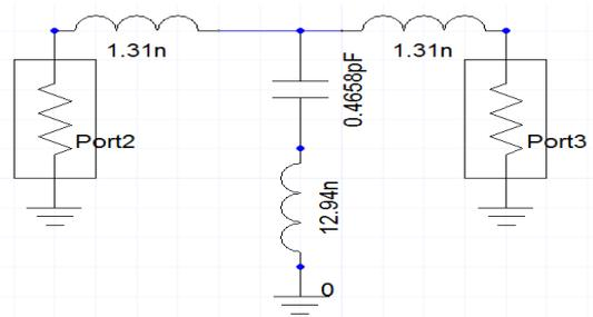
Figure 4 low pass filter m derived in ansoft designer
