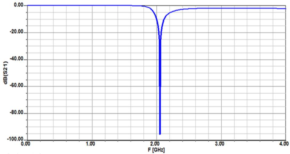
Figure 8. Simulated  $s_{21}$  of m derived low pass filter
