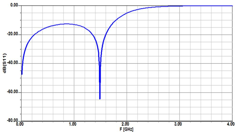
Figure 10. Simulated  $s_{11}$  of constant k low pass filter
