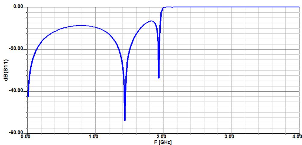
Figure 12. Simulated  $s_{11}$  of constant k low pass filter
