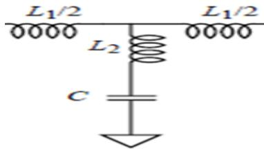
Figure 3 Low-pass m derived filter
