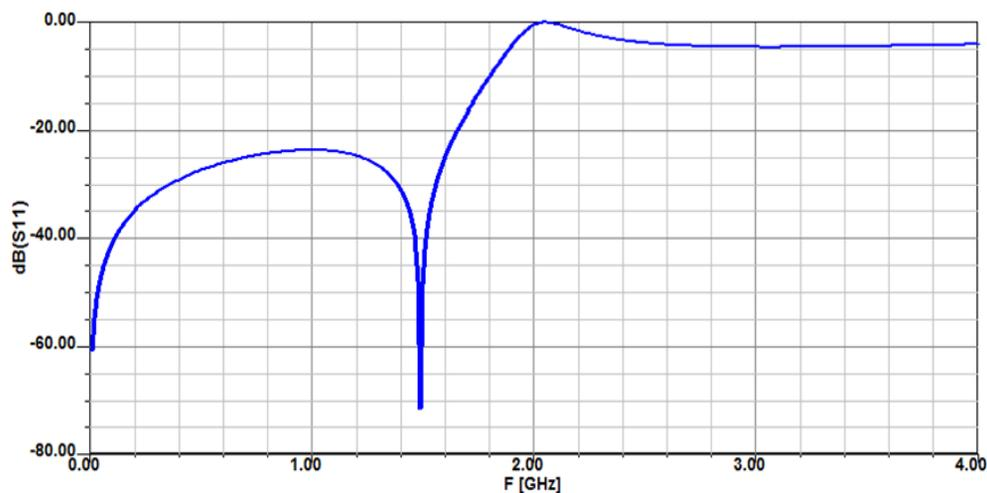
Figure 11. Simulated  $s_{11}$  of m derived low pass filter
