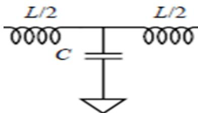
Figure 1. Low-pass constant K filter
