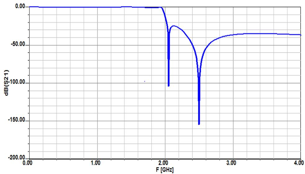
Figure 9. Simulated  $s_{21}$  of composite low pass filter
